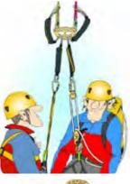
One mountain rescuer is permanently attached to the rigging plate. The second mountain rescuer hangs on a pulley with a self-locking abseiling device. If necessary, he can move away from the dyneema rope suspension up to half the length of the rope carried and ascend again. In case he gets into very steep terrain or a free-hanging situation, he always carries a ascender and a webbing sling (120 cm) with him.
